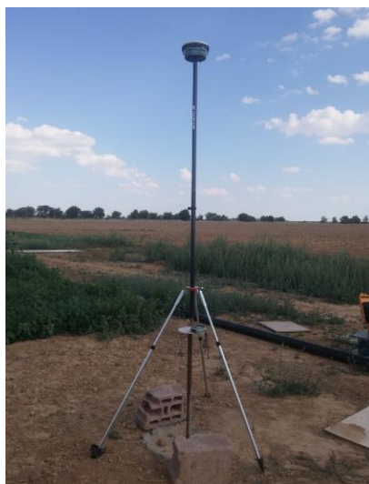
Figure 5. RTK-GPS, Jalon and tripod in operation
