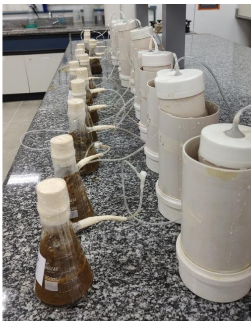
Figure 1. Benchtop bioreactors constructed using 250 mL kitsato flasks, connected to their respective gasometers via silicone tubing.
