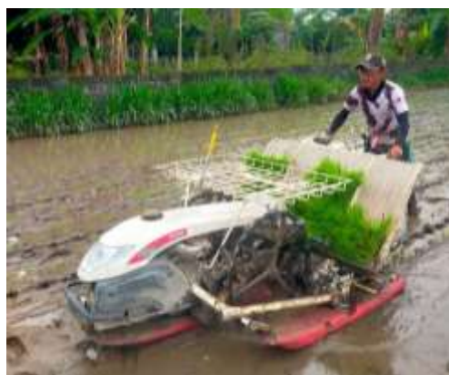
Figure 3. The walking-type rice transplanter
